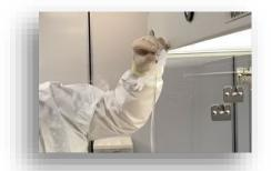
Backstreaming testing — ensures that the lesser-quality outside air does not enter the LAFW's interior workspace. A smoke source is moved along the front access opening, and the certifier visually confirms no smoke breaches the ISO 5 plane as it passes around the perimeter between the external environment and the work area.
